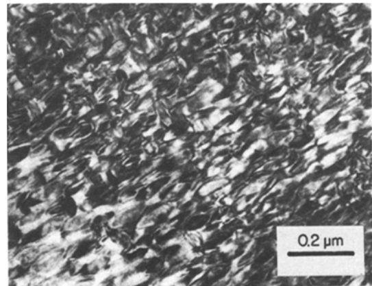
Figure 6 Strain-field contrast around t precipitates in a specimen heat treated at 900^\circ\text{C}/20\text{ h} .
